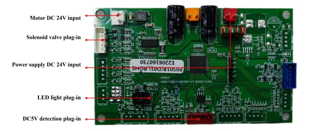
5.7 Mainboard plug-in layout (Left armrest mainboard)
