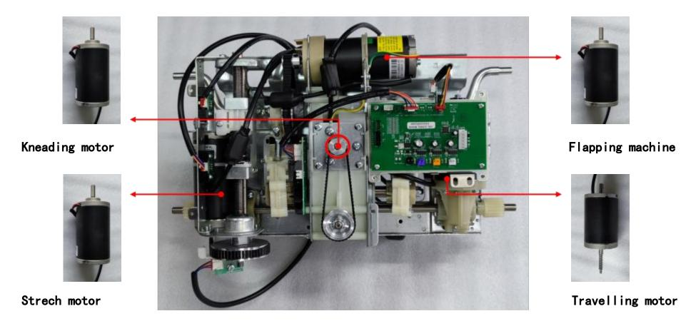
5.10 Back mechanism assembly motor layout (Lower back mechanism assembly)
