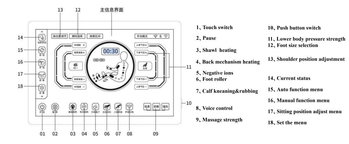
4.2 Manual key function (Refer to the manual for detailed functions)
