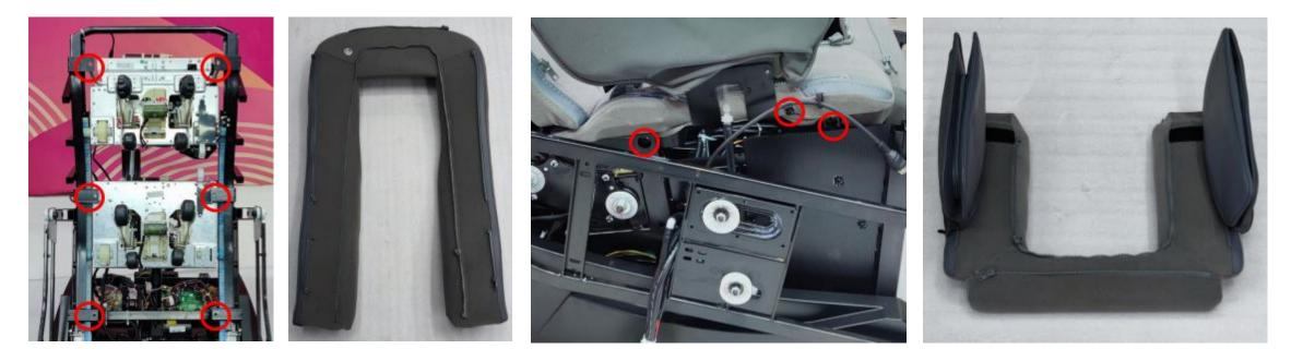
ABCD1. Remove the 62. Remove bracket skin<br/>assembly Figure B3, Remove the left and right screws of Fig. C and the<br/>hand-control fixing screws.<br/>4, Remove the seat frame cover assembly Fig. D.
