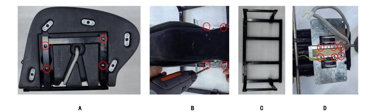
1. Remove the left and right side screws in Figure A. 2. Remove 4 screws as in Figure B. Remove the separation steel frame as in Figure C. 3. Remove 6 screws as in Figure C.
