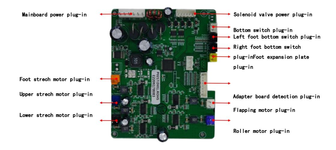
5.9 Back mechanism assembly motor layout (Upper back mechanism assembly)
