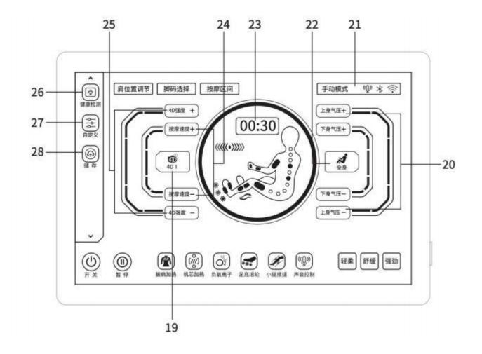
19, Massage technique select **20**, Upper body pressure strength 21, Status display bar 22, Air massage select 23, Time adjust menu 24, Massage speed 25, 4D strength 26, Health check menu 27, Customize menu 28, Save menu
