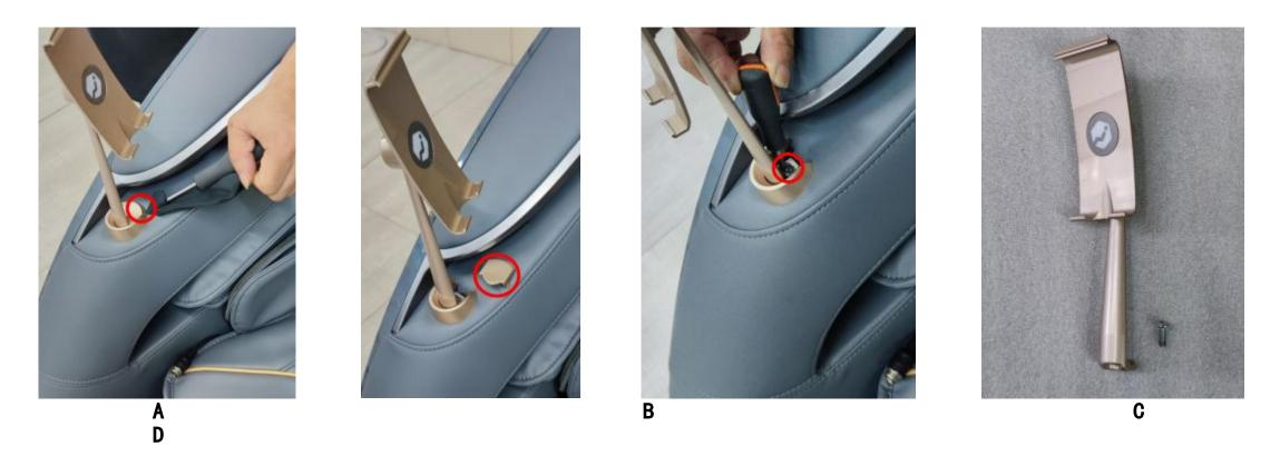
1, With a small word screwdriver with a cloth package, the figure A small decorative removed, as shown in Figure B.
